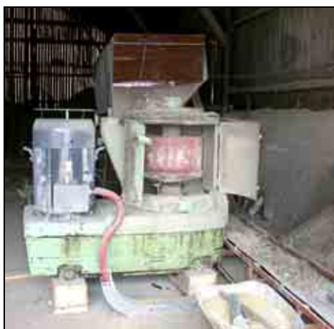
Small granulator for fytomass pellets production. Farmers' cooperation, Argotech Poličná.
