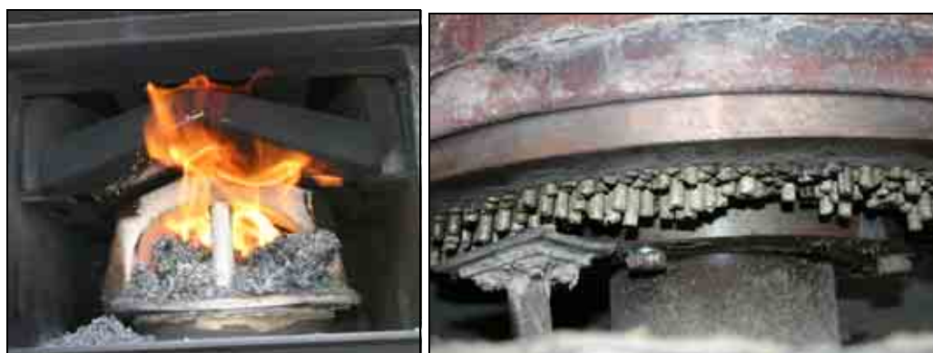
Left: pellets burner. Right: detail of matrix press for bio-pellets production.
