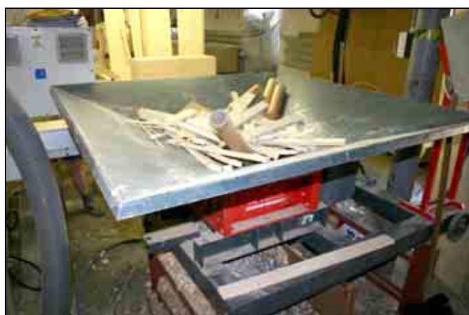
Example of the wood crusher for waste processing in the wood production firm and its use in the kettle for wood chips.
