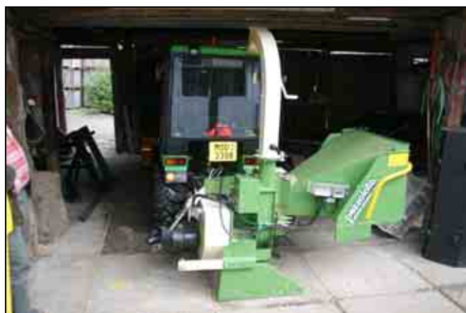
Chipping machine carried and driven by small-tractor. Municipality of Obec Stráž nad Ludinou. Wood chips from the above mentioned chipping machine – Municipality of Stráž nad Ludinou.
